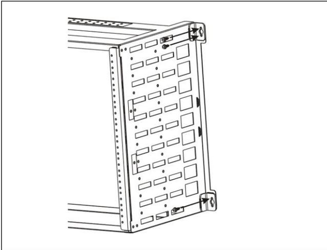
**Figure 6. Mounting screw locations**
